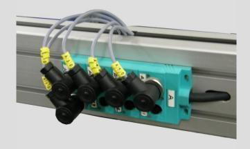
Example of electrical connector (M12x1) for the sheet detectors. It leads the wire that is connected with the exterior of the transfer (harding).
