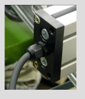
Both pneumatic and electrical connections finish with a connector (which can change according to the customer's guideline) and go out by the end of the pincer-holder bar.
