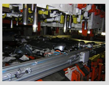
If possible, make a press-transfer process **simulation** at the simulator or with PressLine Simulation, Pressim, etc. programs. This way, we can optimize the *lay-out* (conveyance heights, pincers evolution, etc.) and detect any possible errors and collisions before the *try-out* and production.
